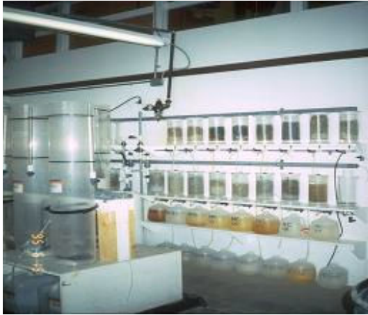
Figure 3. Humidity cells designed for kinetic testing, Zortman Mine.
